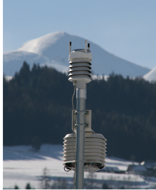
Figure 3: IGFUW automatic meteo-station and EDYTEM temperature sensors deployed on the Niederoeblarn airport (both on the EDYTEM mast)
